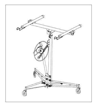
I certify that the Sheet Lifter illustrated above has been tested to confirm the published working load of 68~kg at the standard maximum height of 3.35~m and the extended maximum height of 4.55~m.
