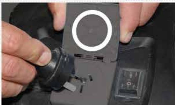
■ Sander power point and on/off switches
