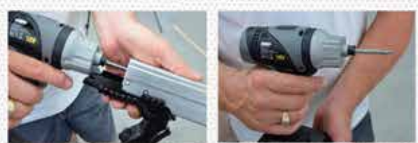
■ Remove conduction assembly ■ Use as screw driver
