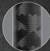
Filament wound carbon fibre tube for non-slip grip
