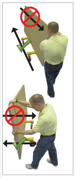
4. As with all carts, when moving the Troll® Cart while loaded, ALWAYS push the loaded cart away from the operator. NEVER pull the loaded cart toward the operator.
